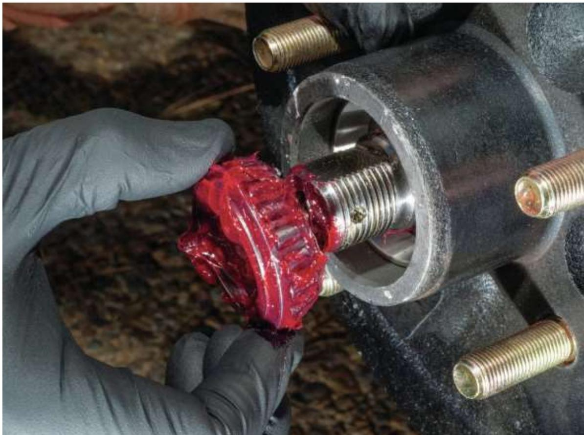
Do up the nut by hand at first, then tighten but not too tight, just check the tightness by spinning the hub, if it feels tight back off one flat of the castle nut and try again. One of the notches on the nut should line up with the split-pin hole. You can then put in your new split-pin making sure you bend it like the way it was when you removed it.
