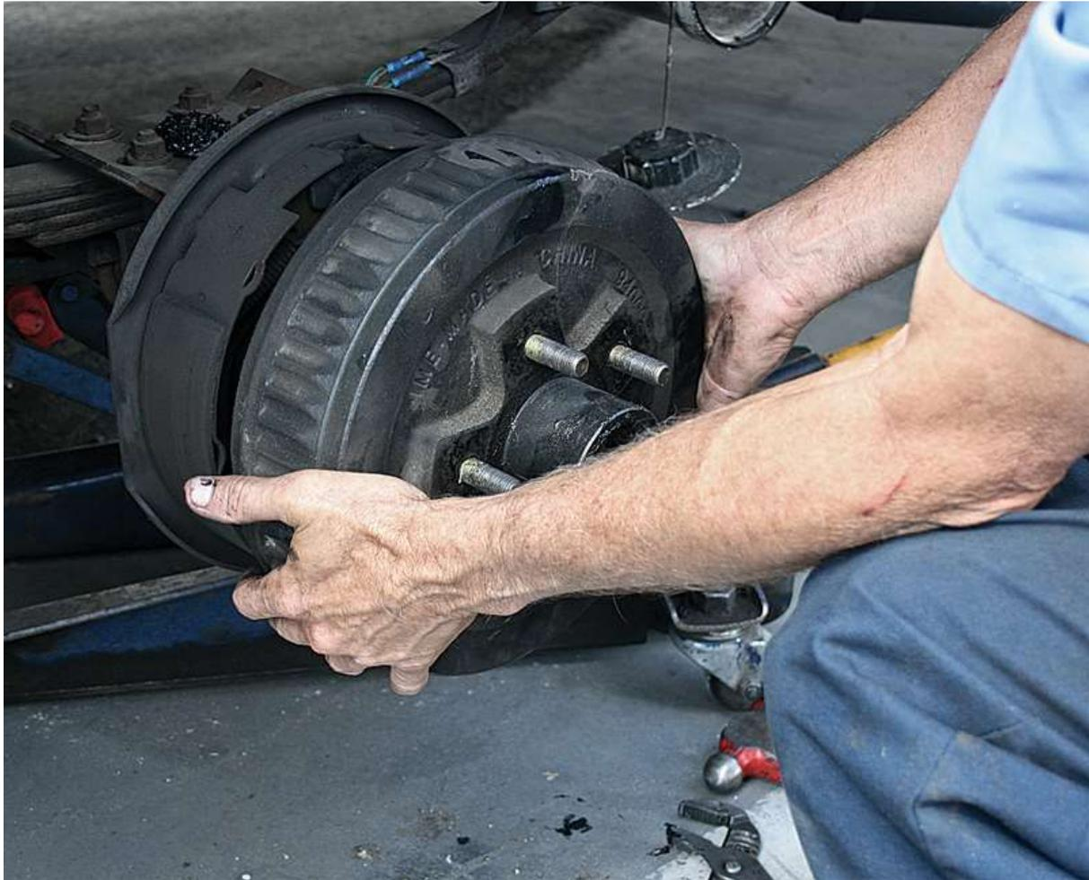
Once removed you can wipe off the grease from the axle stub or spindle with a rag. Place your hub on your workbench and remove the bearings, you'll notice on the inner side there is a seal, just pull it out and the inner bearing should come out easily.
